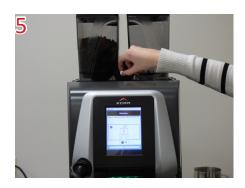
Insert cleaning tablet into the chute on the top of the machine.
