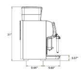
PLEASE NOTE: Power can be installed under or above counter. Please allow 3-4" of space for the plug, especially when placing power above the counter and behind the machine.
